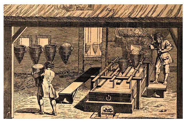
Figure 4. A 16th Century saltworks (from Brownrigg<sup>4</sup>). This image shows the brine being heated and a worker scooping out the crystallising salt and placing it in wicker baskets to drain.
